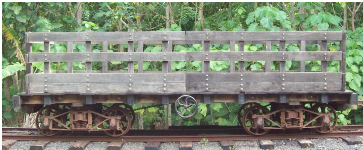
Side Brake Wheel 17 foot Flatcar (sides added) Cane Car
